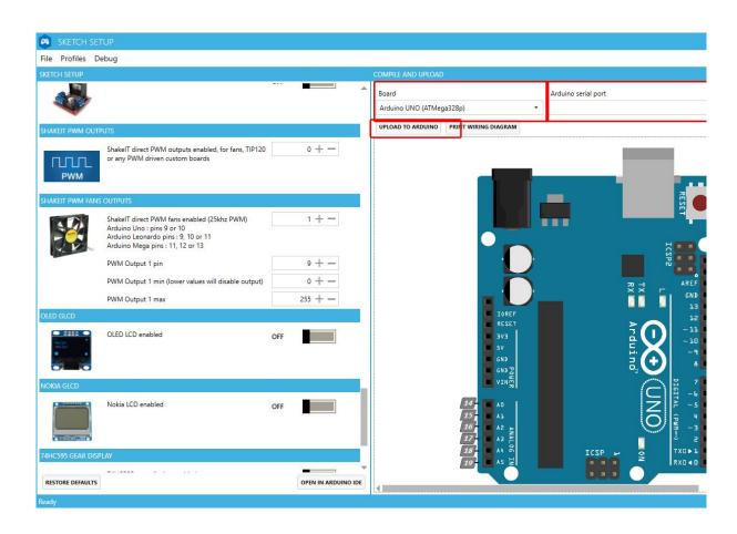
8. When the upload is confirmed close this screen an return to SimHub Arduino screen to select the right COM port. (The selected com port should start with "USB-SERIAL CH340 or Arduino Uno")
