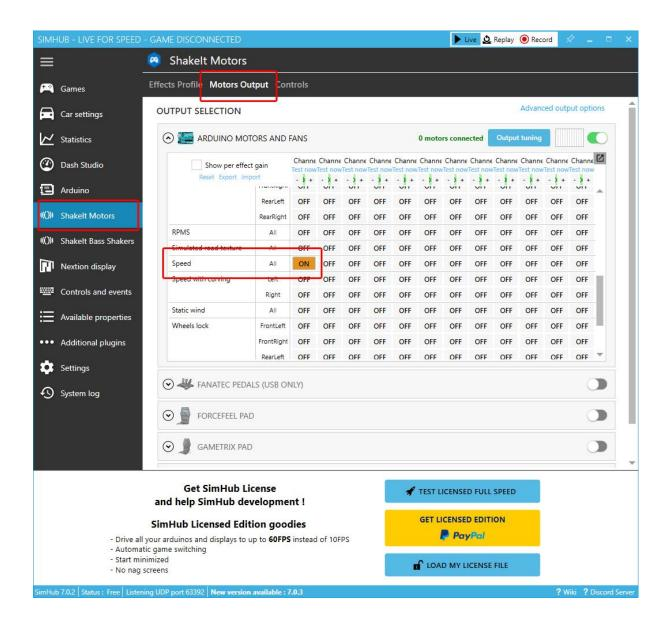
10. Now click on "Effects Profile" and scroll down till you see "Speed". Here you can configure effect setting in the way you want. You can also test the output. If you keep clicking on "Test" and have the power supply connected to your WindSim the fans should spin.
