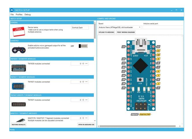
6. On the left side scroll down until you see "ShakeIt PWM OUTPUTS" and set "fans enabled" to 2 (default is 0)
